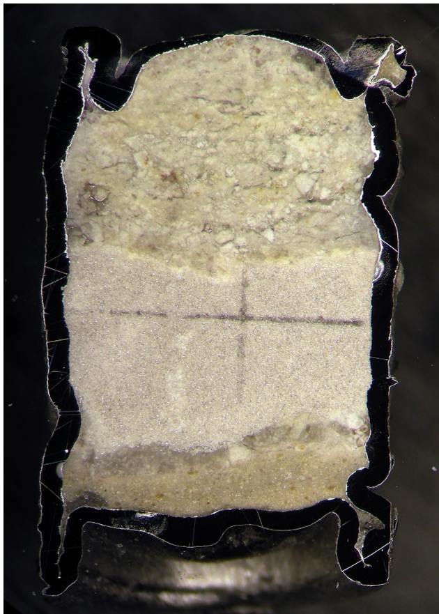
Fig. 3.8-13: Diamond trap capsule after piston cylinder experiment and laser ablation analysis. A diamond powder layer is sandwiched between layers of synthetic eclogite.
